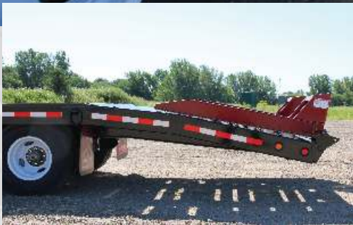
Angle-iron beavertail with 12° to 6° transition to deck.
