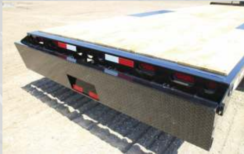
Patented automatic kick-out ramp doubles as under-ride protection.
