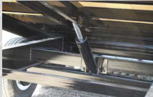
Cushion cylinder controls deck from slamming when loading or unloading equipment.
