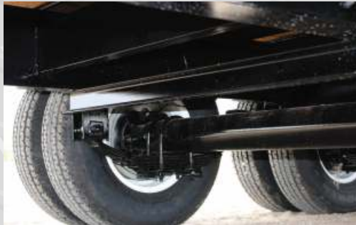
Single-wheel tri-axle. 6K axles with spring-ride suspension.
