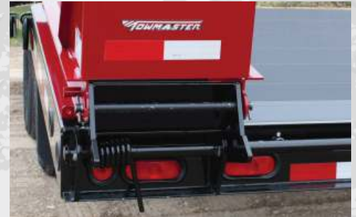
One-way spring-assist ramps and grommet mounted LED lights.
