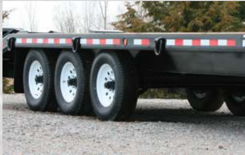
Single-wheel tri-axle. 6K axles with spring-ride suspension.
