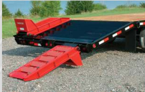
Angle-iron beavertail and ramps provide excellent traction for loading and unloading.
