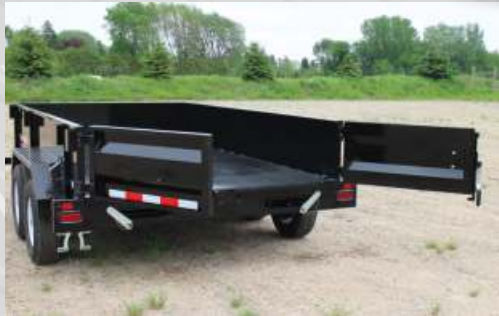
Barn-door style rear gate can be attached in place with a cable to keep them out of the way when lifting dump bed.
