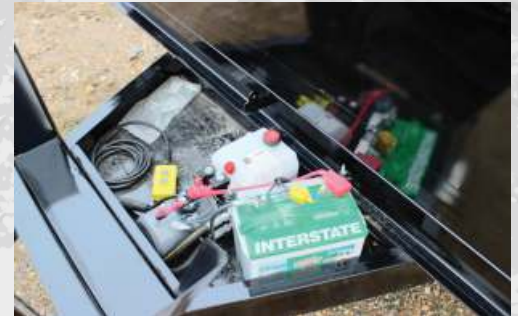
Built-in storage box houses hydraulic system with room for chains, straps or tools.
