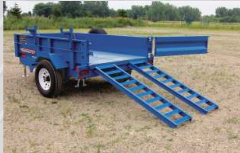
Optional ladder-style ramps for loading equipment, stored above fender.
