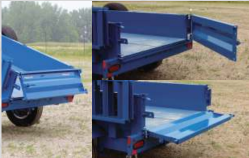
Tri-swing rear gate opens to the side, down from the top, or swings open from the bottom.
