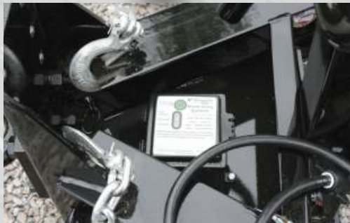
Sealed battery break-away system charges while plugged into the tow vehicle and can be checked at the press of a button.
