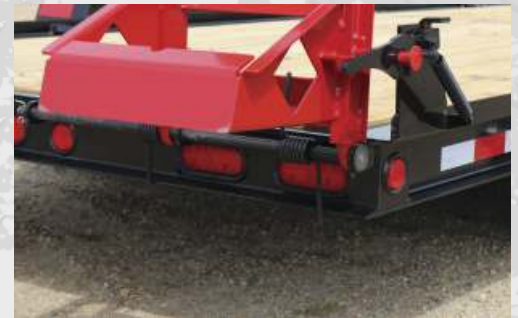
Strong, channel side ladder-style ramps with patented Auto-Latch® ramp hold-ups.
