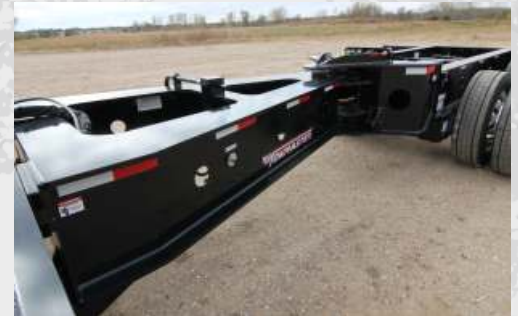
Heavy-duty articulating frame.
