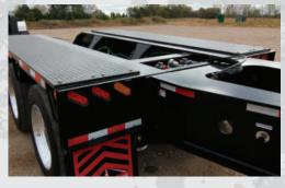
A stronger trunnion section allows the use of a flip-axle or booster to better distribute the load.
