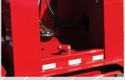
Hydraulic cylinders are encased in the uprights Air Pin design locks gooseneck to deck. The
