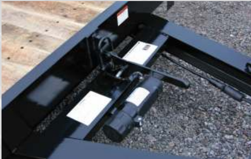
Positive locking (over-center) latch system keeps deck secured to the frame.
