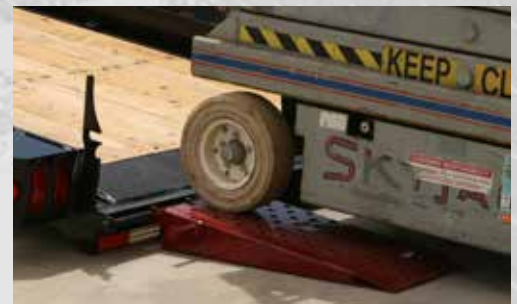
The "SL" (Scissor Lift) option included ramps to lower the loading incline.
