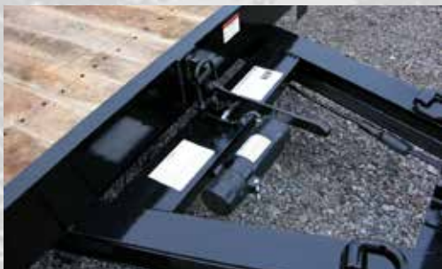
Positive locking (over-center) latch system keeps deck secured to the frame.
