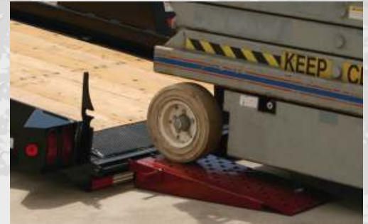
The "SL" (Scissor Lift) option includes ramps to lower the loading incline.
