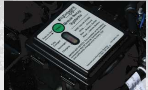
Sealed battery break-away system charges while plugged into the tow vehicle and can be checked at the press of a button.
